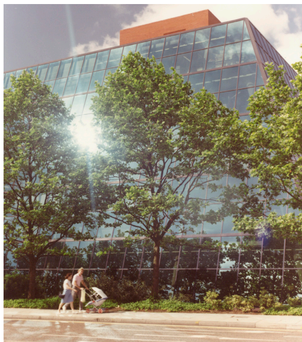
Figure 41: Solar dazzle reflected from a glazed façade
