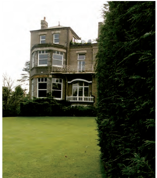
Figure 31: A dense belt of coniferous trees should be treated as an obstruction to sunlight
