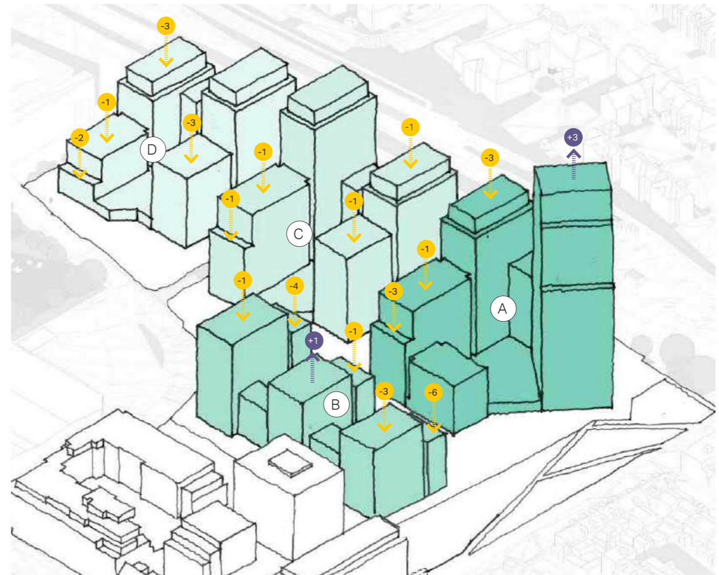
Massing 5 - Sketch aerial view showing design development and height adjustments made following Pre-application Workshop 03
