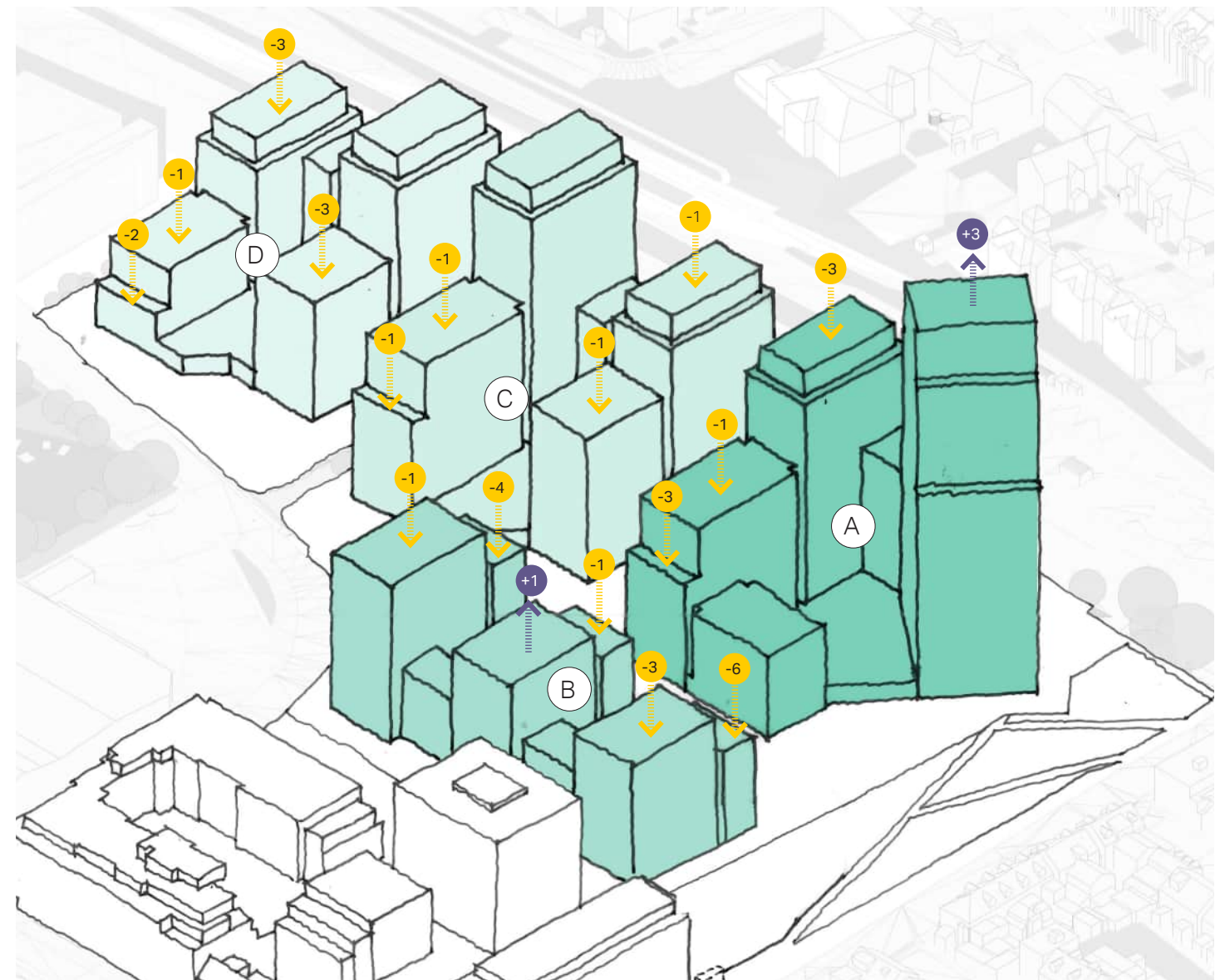
Figure Massing 6.13 - Sketch aerial view showing design development and height adjustments made following Pre-application Workshop 03
