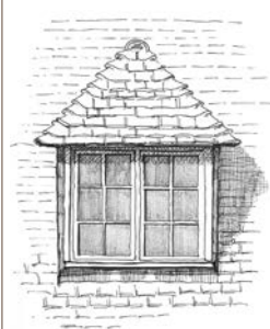
▼ A hipped roofed dormer and a flat lead roofed dormer.
